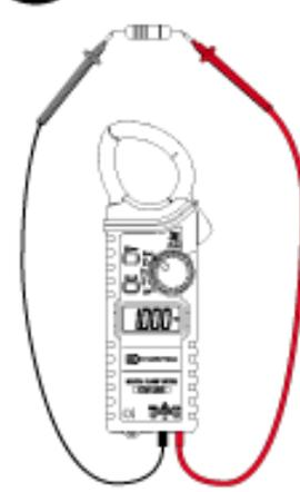
Press the trigger to open the current sensor and clamp the one conductor under test.
